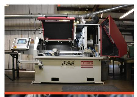
The VA-L 560NC is a circular cold saw specifically geared toward aluminum and is suited for Kyser's specific production needs.
