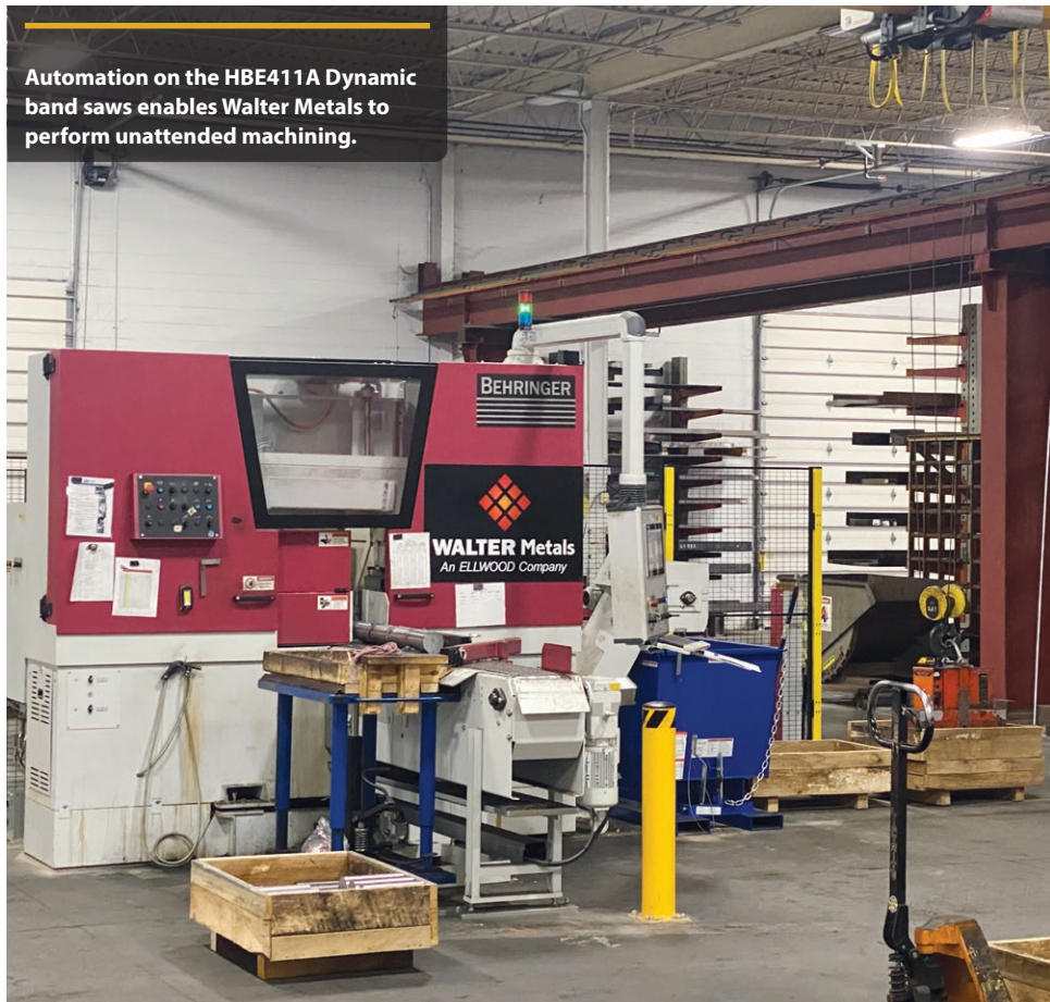
The Behringer automatic band saws reduced material handling time by 50 percent at Walter Metals to eliminate bottlenecks.
