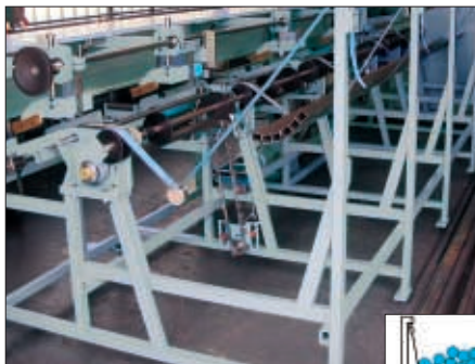
The Bundle Loading Magazine is designed for the automatic loading of round, square or rectangular shaped material with an additional separation device for thin-walled tubing.
