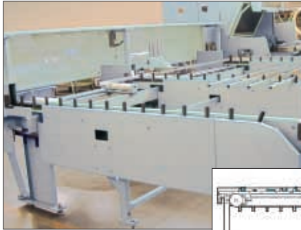
The KLM Flat Magazine can be used for the automatic feeding of a variety of profiles.
