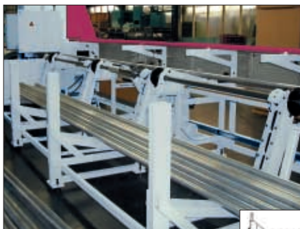
Lift Loading Magazines for the automatic loading of larger dimensioned tubes, square or rectangular shaped material.
