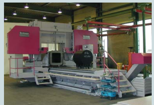
BEHRINGER HBP 1300 Gantry with traversable saw frame.
