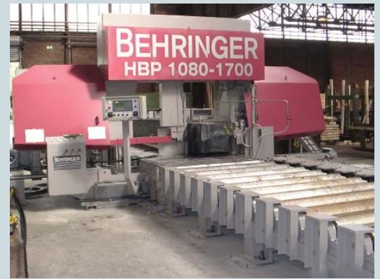
BEHRINGER HBP 1800-1700 width heavy-duty roller conveyor.
