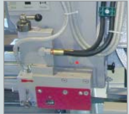
Combined saw blade roller and carbide guides
