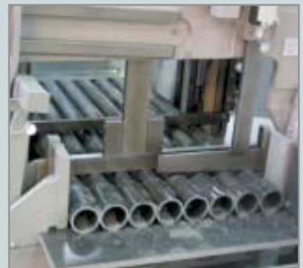
Vertical clamping unit for reliable clamping of material layers
