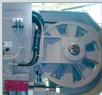
Dual wheel bearings for reliable saw blade running even under maximum loads
