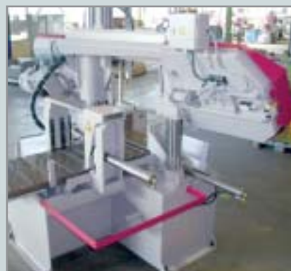
The electronically controlled feed gripper quickly and precisely positions the material for cutting
